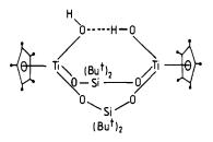
The hydrogen bridge increases the coordination number of O(1) and results in a long Ti(1)-O(1) bond, 187.2(2) pm. Normally the elimination of a water molecule would be expected, but in this case steric factors presumably prevent further reactions of the OH groups.
