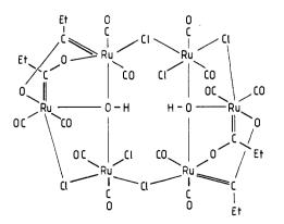
The complex is prepared by the reaction of  $Ru(C_3H_5)$ -Cl(CO)<sub>3</sub> with CH<sub>2</sub>=CH<sub>2</sub> in benzene. The Ru-OH distances are 216 pm (av).
