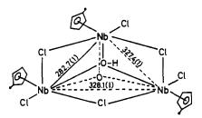
Each edge of the triangle is bridged by a chloride while a  $(\mu_3$ -O) and a  $(\mu_3$ -OH) triply bridge opposite faces of the Nb<sub>3</sub> triangle. Terminal C<sub>5</sub>H<sub>4</sub>Me and Cl ligands on
