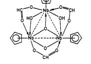
In this  $d^1$  niobium compound the metal atoms are located at the vertices of an almost regular triangle with short Nb–Nb distances (314 pm, average).
