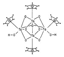
The two terminal hydroxo ligands are attached to the wing-tip Ta atoms. Direct metal-metal bonds are not required to interpret the structure.
